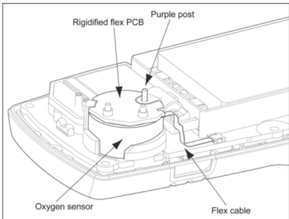
2. Note the placement of the PCB to ensure it is replaced correctly. Remove the two screws on the PCB.
